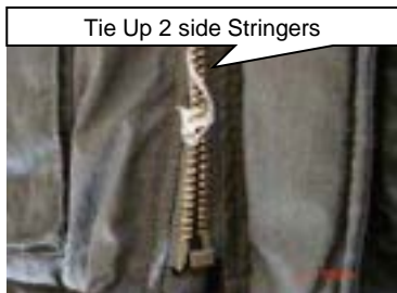
Open up the zipper to prevent twist force gathering at tape ends.
