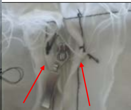
The garment fabric is sewn down to keep away from contact with the slider.
