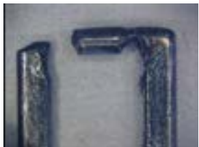
Corrosion took place on zinc die-cast slider pull under the strong chemical treatments.
