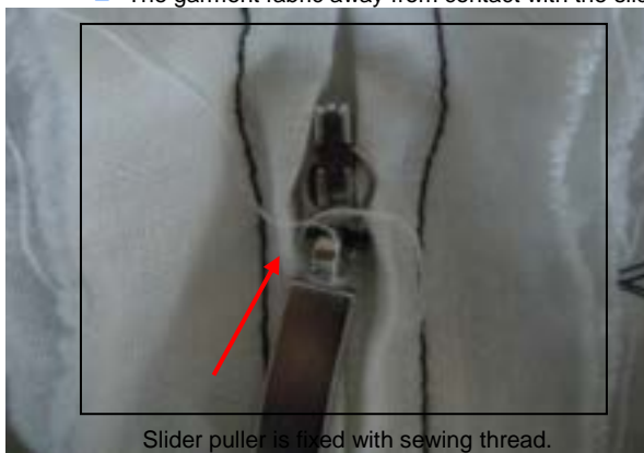
The garment fabric is sewn down to keep away from contact with the slider.
