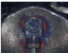
Slider damage due to the dissolving of zinc alloy slider under strong chemical treatments in garment processing.
