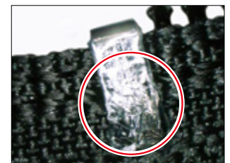
Coil zipper (P-TOP) damage example
