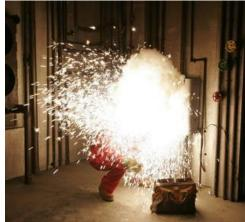
Kincetries Test #09-2156 &kA, 26 cycles YKK Level 1A Front & Pocket zipper snap hook
